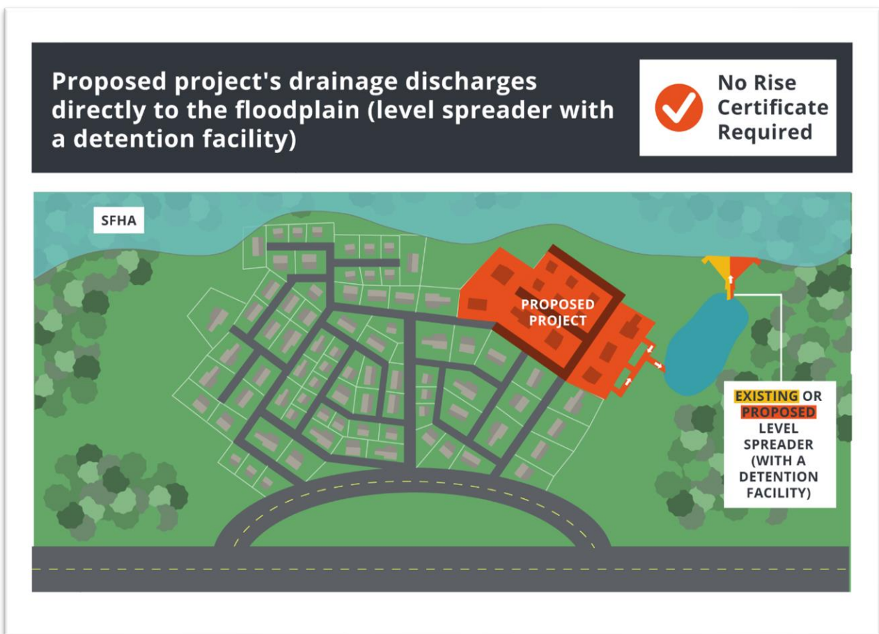
Figure 18: No-Rise Certificate requirements when discharging stormwater through a level spreader without a detention facility that outfalls in the SFHA.
