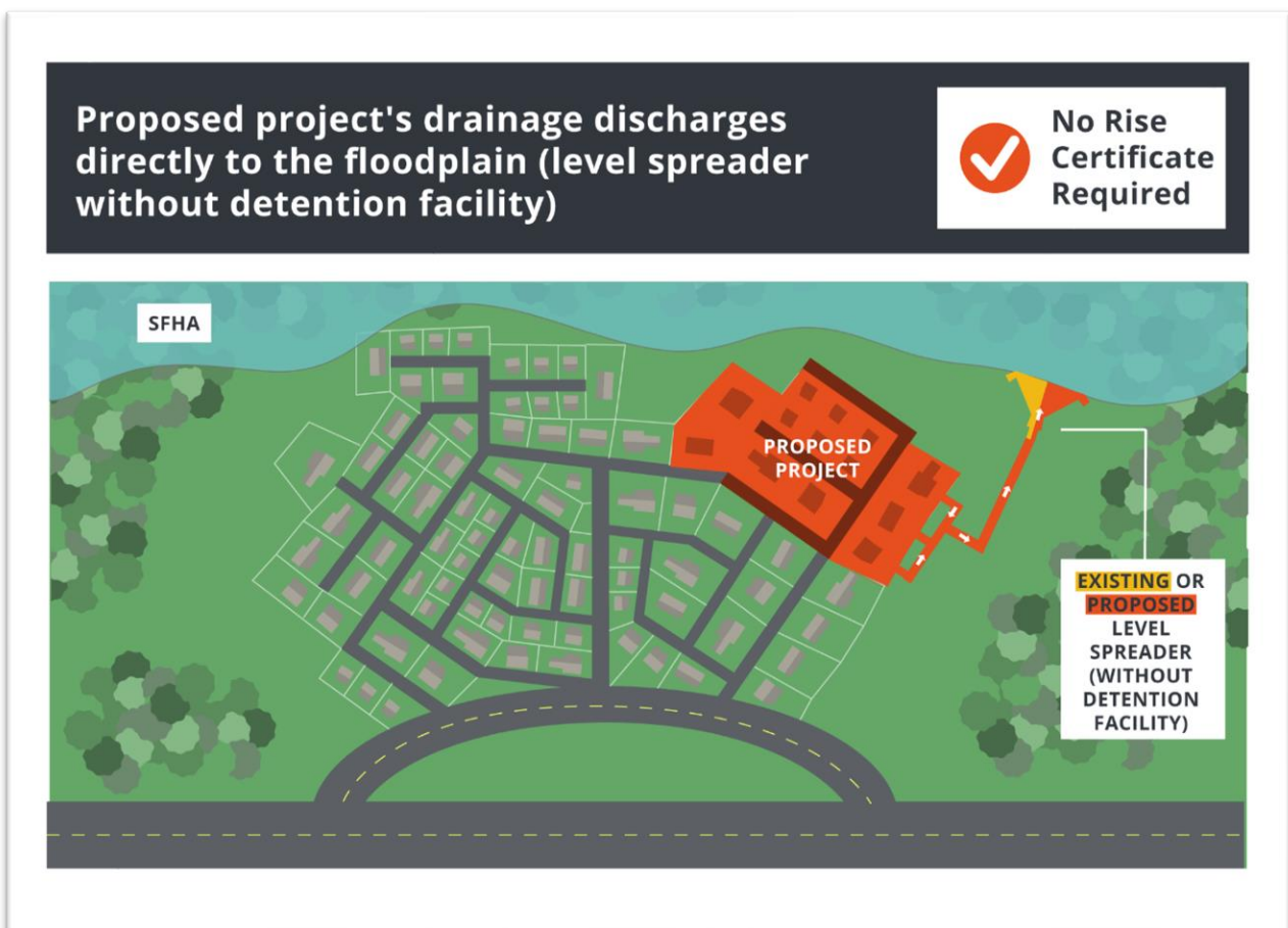
Figure 17: No-Rise Certificate requirements when discharging stormwater through a level spreader without a detention facility that outfalls in the SFHA.
